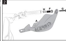
Fix the handguard (A) to the handlebar using the expander (F), the insert (H) and the screw (G) as shown in the figure.
