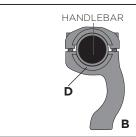
Use the spacer (D) for handlebars fatbar 28mm-1+3/32 inch.
