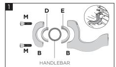
Mount the bracket (B) on the handlebar using screws (M) and if necessary use the spacers (D) or (E).
